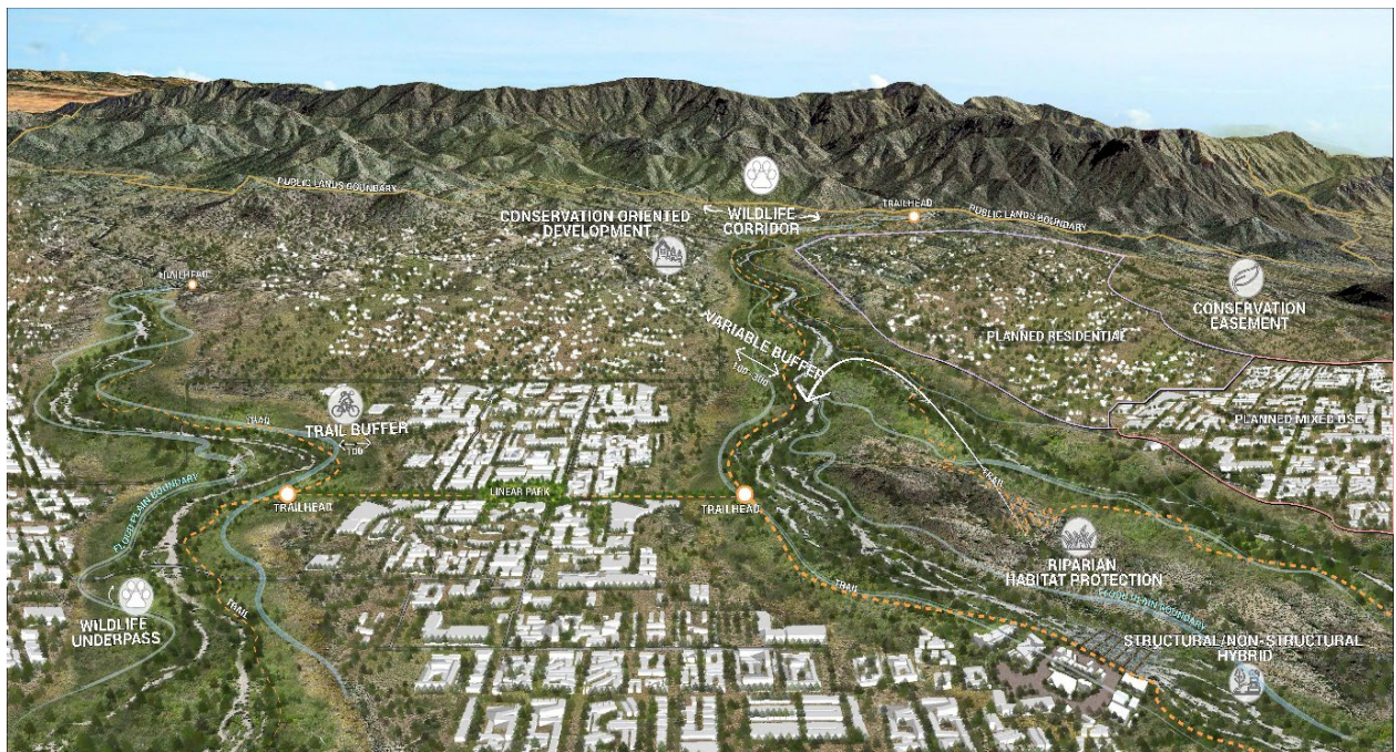
Figure 14. Conceptual Plan for the White Tank Mountains in the west valley, includes use of GI and LID technologies with hybrid natural and structural floodways. Developed by Logan and Simpson
