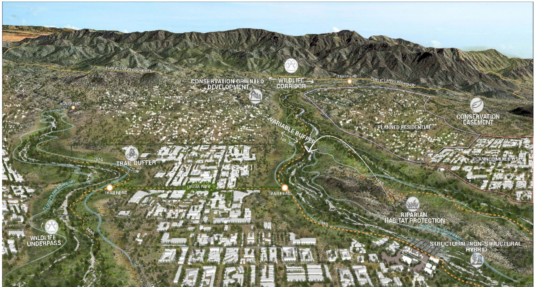
FIGURE 14: Conceptual Plan For The White Tank Mountains In The West Valley, Includes Use Of GI and LID Technologies With Hybrid Natural and Structural Floodways.
