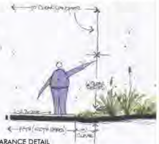
PRIMARY TRAIL CLEARANCE DETAIL
